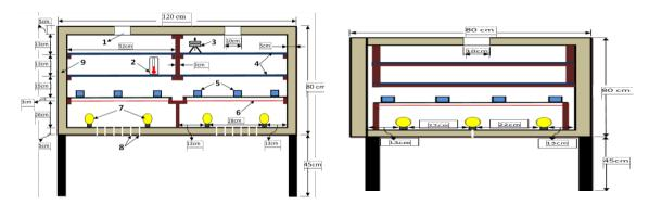
in this study, while Figure 2 shows the dimensions of a side incubator used in this study.
